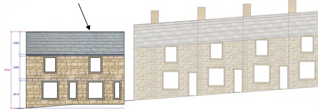
Front Elevation Clive Street Easier construction of level roof plane, windows and doors on same level; pattern still replicates street scene.
